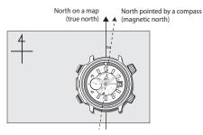
Declination correction is a correction method to adjust the compass of the watch to indicate true north as indicated on a map by setting the declination value of the location where you wants to find compass direction on the watch previously. On this watch, declination of 0° to 59° east and west can be set by 1°. You can use the results of geomagnetism survey published by governmental or other organizations.
